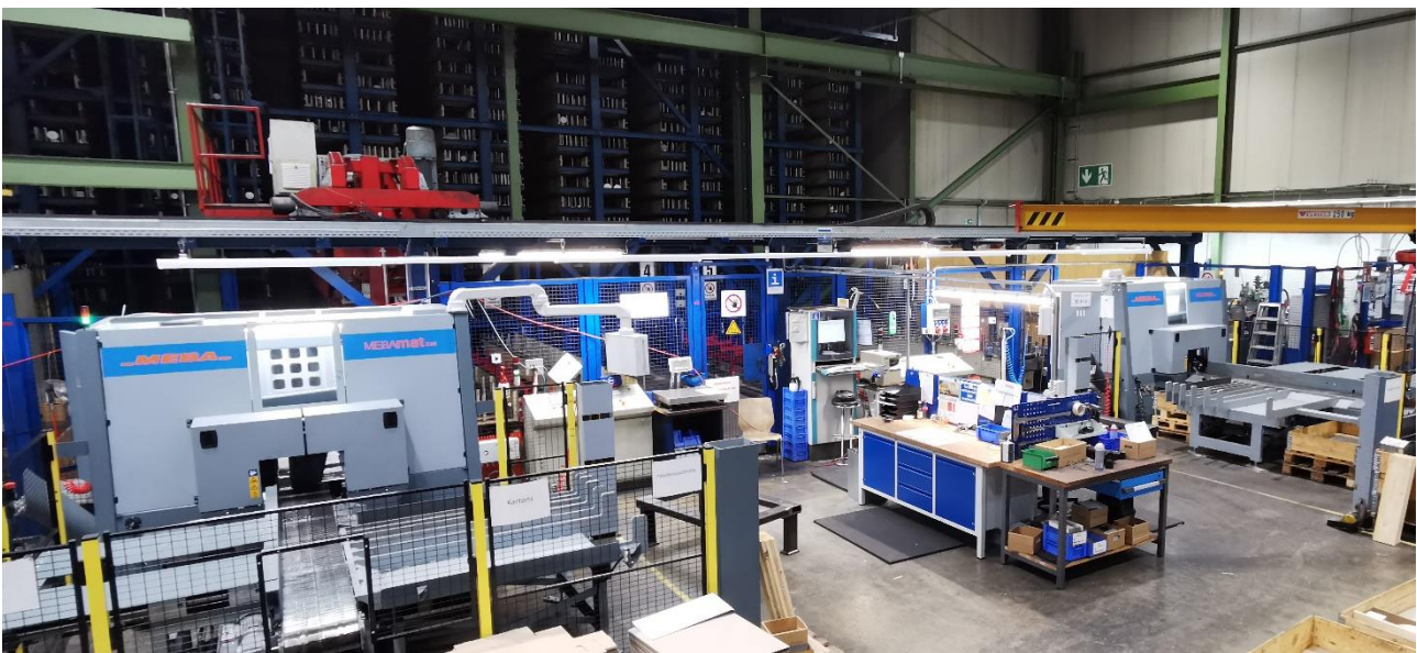
automated and digitized sawing system with high-bay connection
