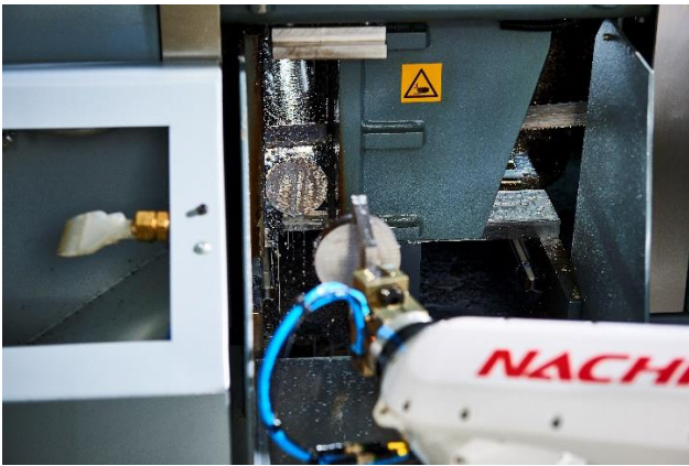
Removal of the sawn parts
